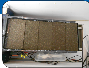
Deck-Air® Vent Installed on Test Roof Deck
