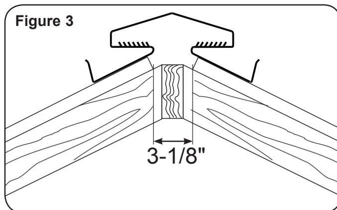
inches inside the overall length of the vent as measured in Step 1 and Step 2. The hole is best cut with a circular saw taking care to set the depth of the blade to avoid cutting the rafters or ridge pole.
